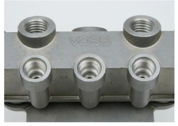
Fig. 11: Clean and correct connecting bores
