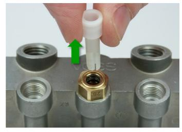
Fig. 16: Pulling out the assembly plug
