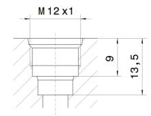
Fig. 5: Profiled bore for M 12 x 1 thread
