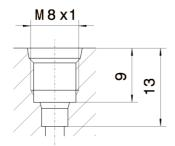
Fig. 3: Profiled bore for M 8 x 1 thread
