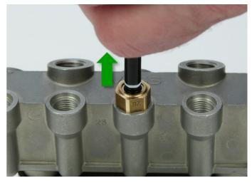
Fig. 23: Pulling back the polyamide tube
