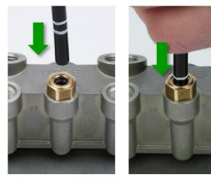
Figs. 19+20: Pushing-in the polyamide tube
