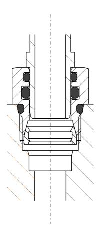
Fig. 25: Schematic diagram for a male gauge
