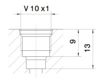
Fig. 7: Profiled bore for V 10 x 1 thread
