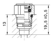
Fig. 21: Push-in depths and dimensions NS 4 and NS 6
