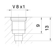
Fig. 6: Profiled bore for  $V 8 \times 1$  thread
