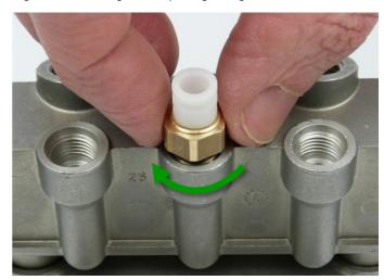
Fig. 13: Screwing in the assy manually
