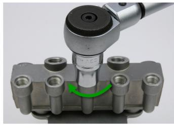
Fig. 14: Tightening with a torque wrench
