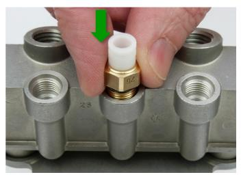
Fig. 12: Positioning the assy at right angles
