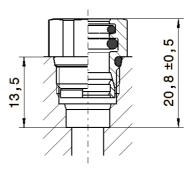
Fig. 22: Push-in depths and dimensions NS 8
