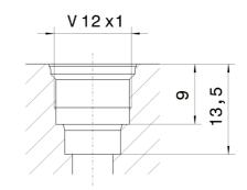
Fig. 8: Profiled bore for V 12 x 1 thread
