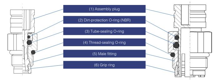
Fig. 1: Components of the assy VOSS quick connect system 203 (left: NS 4, right: NS 8)
