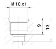
Fig. 4: Profiled bore for  $M 10 \times 1$  thread
