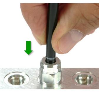
Fig. 14: Pushing-in the polyamide tube to the tube stop
