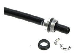
Fig. 21: Detached spacer and cut grip disc
