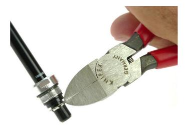
Fig. 19: Cutting the grip disc
