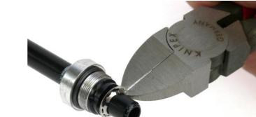
Fig. 20: Cutting the grip disc at the opposite position
