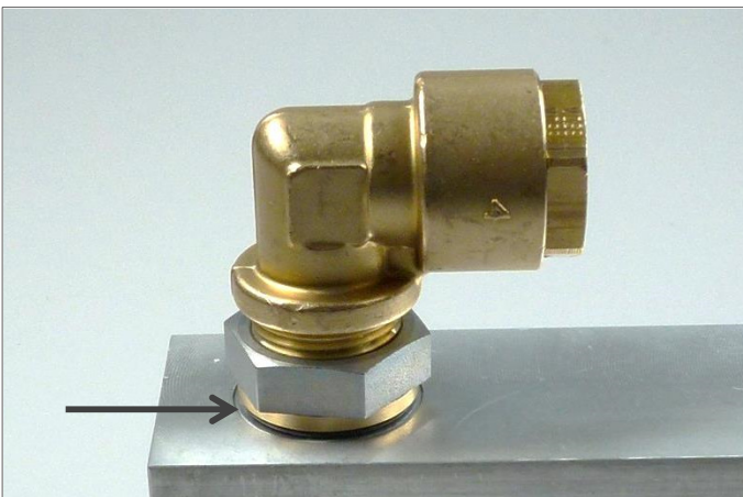
Fig. 7: Screw in the elbow connector until the O-ring reaches the contact surface
