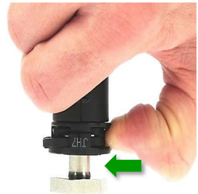
Fig. 24: Pushing in retaining clip 241 N-SL
