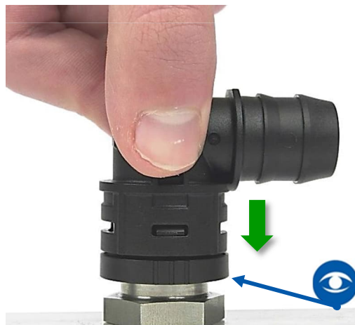
Fig. 29: Plugging in coupling 270 as far as it will go
