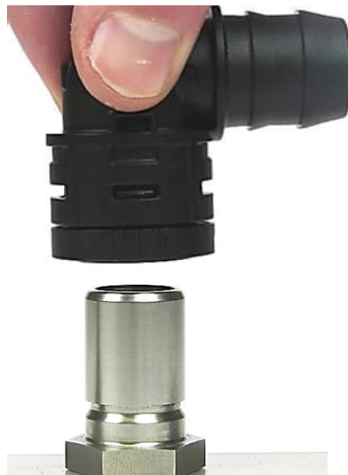
Fig. 23: Centered placement of coupling 270 above male connector
