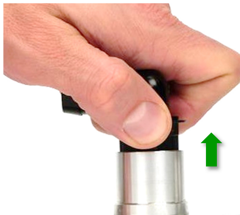
Fig. 30: Pulling out the plug 271
