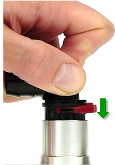
Fig. 12: Inserting plug 271 DL into connecting port
