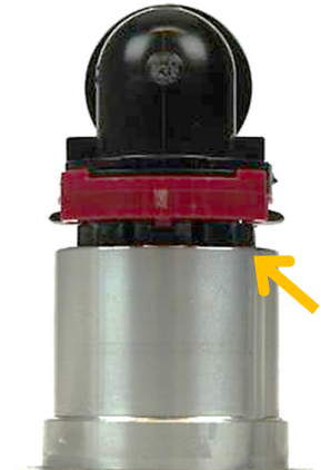
Fig. 14: Incomplete assembly plug 271 DL : blocked Double Lock
