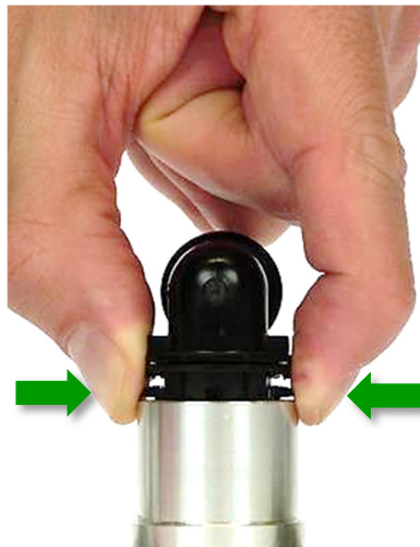
Fig. 28: Squeezing of the locking element of plug 271
