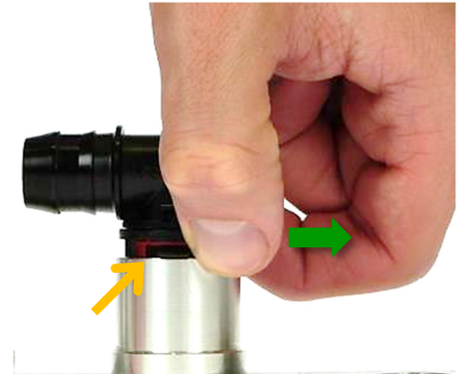
Fig. 23: Pulling away the Double Lock
