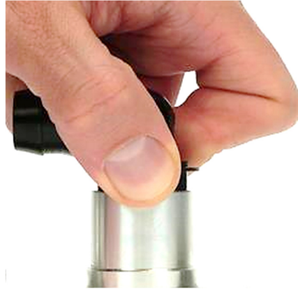
Fig. 26: Grasping the locking element of plug 271
