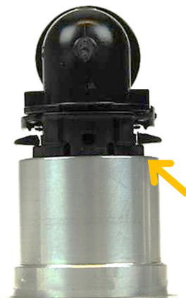
Fig. 13: Incomplete assembly plug 271
