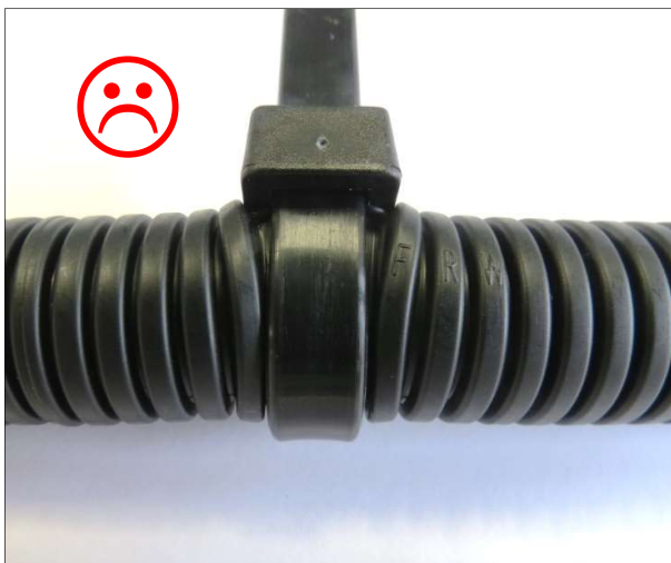
Fig. 5: Incorrect use of a plastic zip tie
