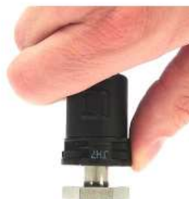
Fig. 37: Activated secondary lock (subsequent assemblies)
